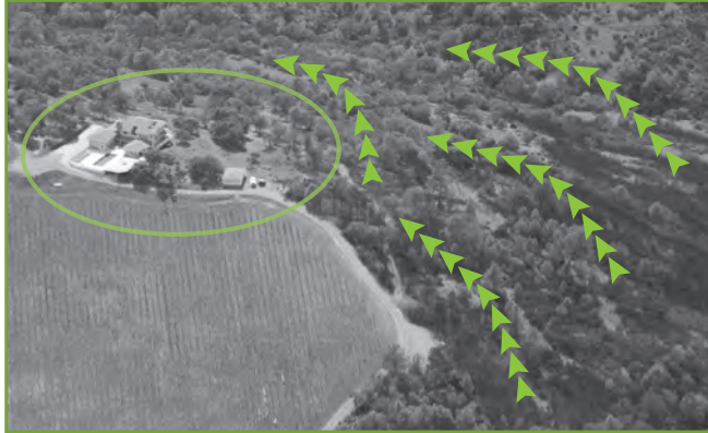
Aerial view showing path of Soda Fire. Arrows show the pathway of the fire and defensible space protected this house
